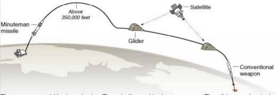
The weapon would be launched on a Minuteman missile, which travels at altitudes above 350,000 feet. The missile would release a hypersonic glider that would receive updates from satellites as it travels toward the target. The glider may be designed to release a 1,000-pound conventional weapon that could penetrate deep into the earth.
